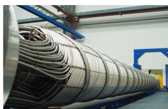
8 Sets of Coil-Wound Heat Exchanger in Rectisol Process System for Coal to Hydrogen Complex
